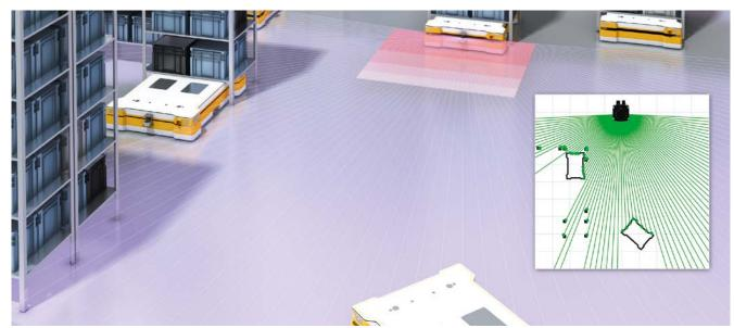
Localization and collision avoidance in automated warehouses.
