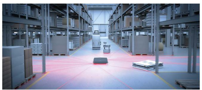
Simultaneous localization and mapping (SLAM).
